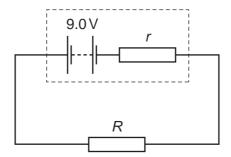
A charge of 6.0 C flows through the resistor in a time of 2.0 minutes causing it to dissipate 48 J of thermal energy.
